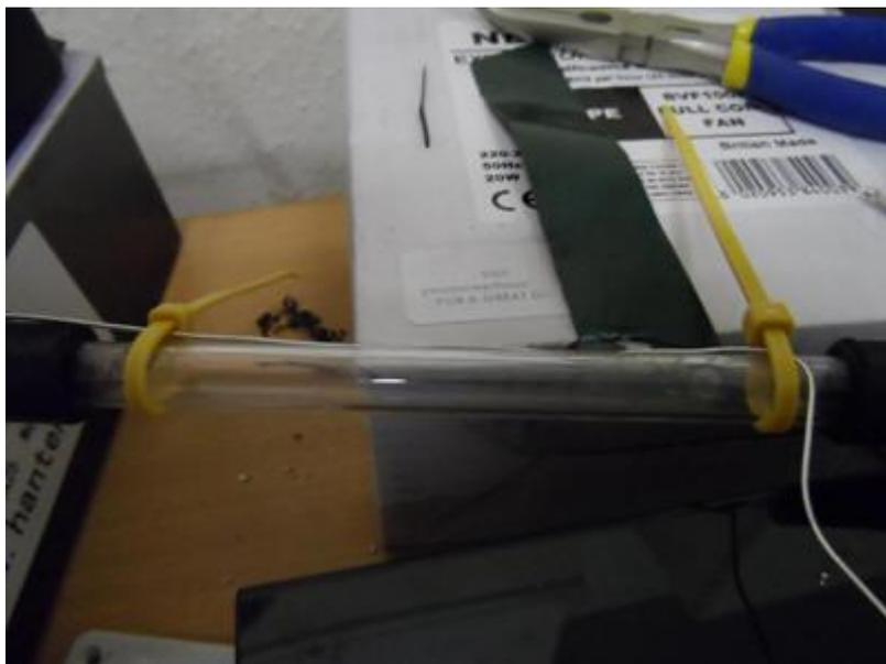
The ionisation wire arrangement. This gives a more even distribution and will not cause as much interference with the winding.
