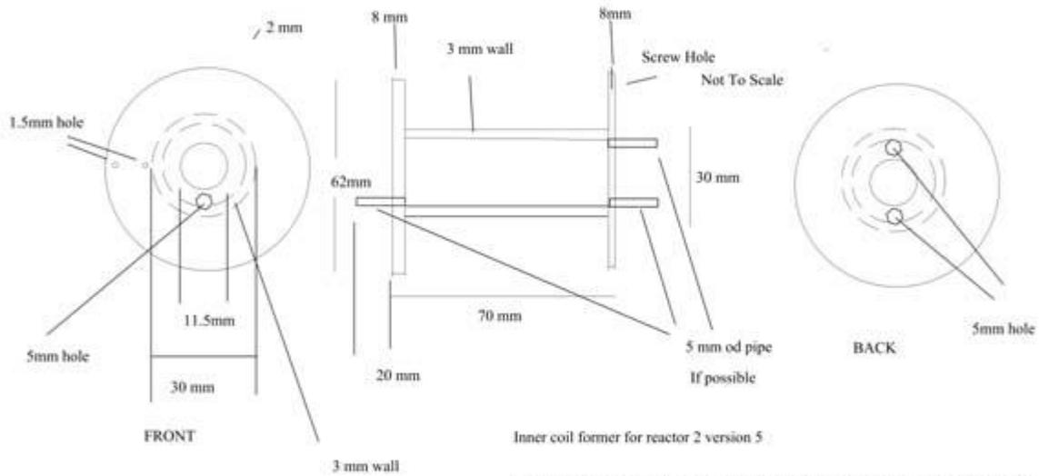
Inner coil former for reactor 2 version 5
